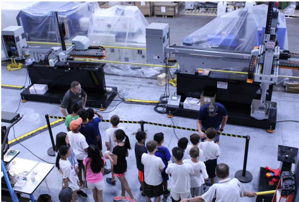
PHOTO 3: ARI's Business Unit Manager Tim Lavigne (left) answers questions while Service Manager Tyler Alcock shows students how to use the robot's control. The robot on the left is a MaxA05-1000P and the robot on the right (the larger robot) is a MaxBW15-1700P. Both are 3-axis robots.
